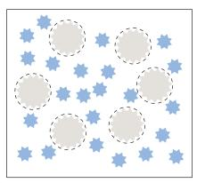
Figure 4: A precipitate on the surface of the cement particles preventing water reaching them
