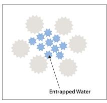
Figure 2: Flocculating cement particles trapping the mix water
