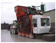
Most modern block making plants in the UK are highly automated and the block making machine is stationary. Earth-dry concrete is fed to the mould where it is vibro-compacted onto steel, timber or plastic pallets.
