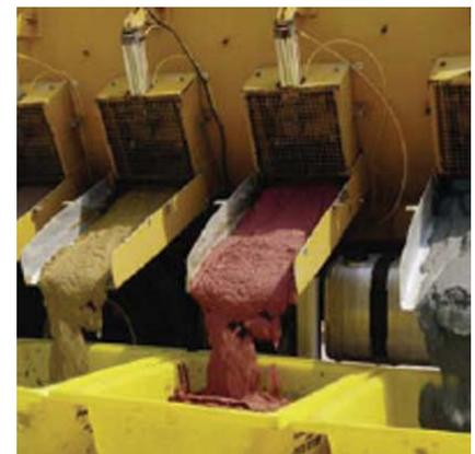
one vehicle. Some of these are designed as demountable units, so that the delivery truck may be used as an ordinary tipper vehicle when required by removing the mortar mixing/delivering modules. Some designs allow agitation en route, with others this is not possible.
