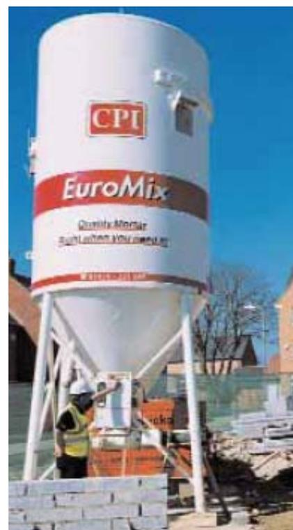
the silo. Because the throughput time for these mixers is very low, in the order of only a few seconds, the design of the mixer screw and chamber is critical. These mixers perform very effectively in practice and the dry mortars require careful mix design to take account of the reduced mixing energy input during the brief mixing process.
