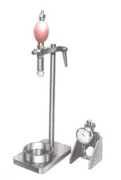
Dropping ball apparatus used in the testing of fresh mortar
