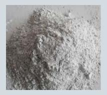
The use of ground granulated blastfurnace slag (ggbs) and fly ash in mortar has increased in recent years. Records indicate that blastfurnace cement was used for the mortar during the construction of the Empire State Building in the 1930s. Fly ash has been used as a constituent material of mortars for over thirty years, and in the case of some of the bagged proprietary mortars for an even longer period.
