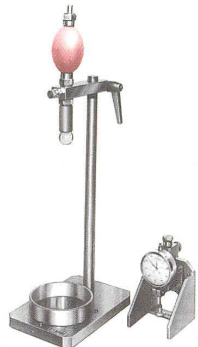
.95 Figure 1: Dropping Ball Apparatus
